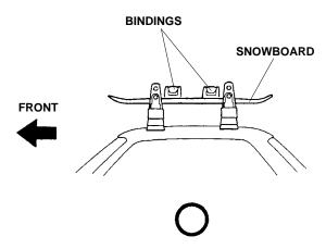
11. If the bindings cannot be positioned between the front and the rear attachments, install the snowboard with a binding behind the rear attachment as shown.
